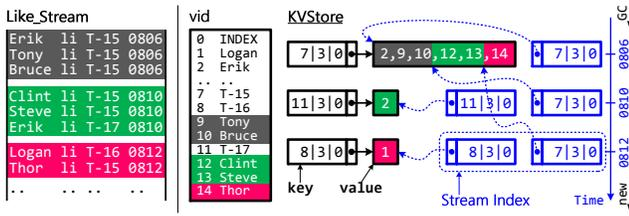
Fig. 8: The design of stream index in Wukong+S.
