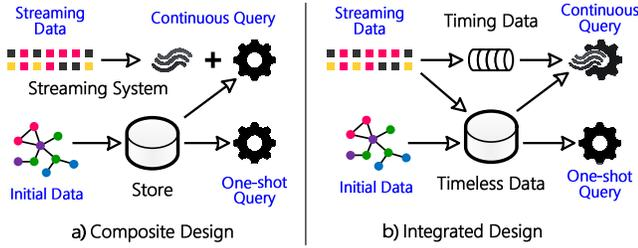
Fig. 3: A comparison between composite and integrated design.
