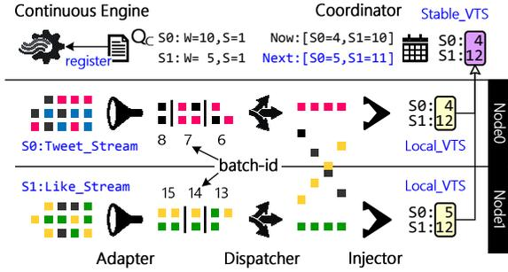
Fig. 10: Distributed stream injection and punctual query trigger.
